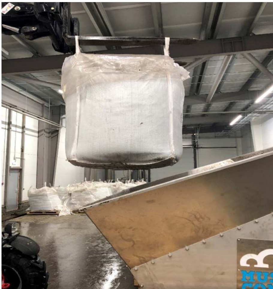
Above: Not the ideal situation but if there is no clean space available you can unload the casing soil from the big bags directly into the machinery.
